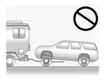
All-wheel-drive vehicles must not be towed with two wheels on the ground. To properly tow these vehicles, they should be placed on a platform trailer with all four wheels off of the ground.
