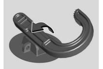
1. Insert one side of the load floor hook into the holder.
