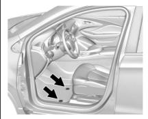
The driver side floor mat is held in place by two retainers.
