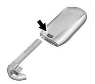
1. Press the button on the transmitter to access the key.
