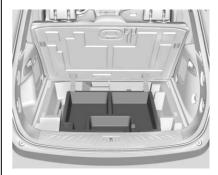
The cargo management system is used to store items in the cargo area under the load cover.
