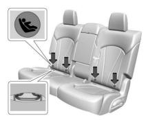
The lower anchors are behind the horizontal openings in the seat cushion trim located below the anchor label.
