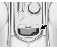
There is a small bin directly in front of the center console. On some models, the bin has a cover. Use the handle to open the covered bin.
