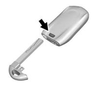
Press the button on the RKE transmitter to remove the key.
