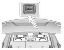
Press any liftgate button or the touch pad while the liftgate is moving to stop it. Pressing again restarts the operation in the reverse direction. The touch pad on the liftgate handle cannot be used to close the liftgate.
