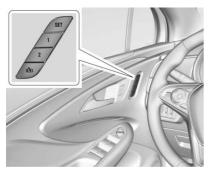
If equipped, memory seats allow two drivers to save and recall their unique seat positions for driving the vehicle, and a shared exit position for getting out of the vehicle. Other feature positions may also be saved, such as power mirrors and power steering wheel, if equipped. Memory positions are linked to RKE transmitter 1 or 2 for automatic memory recalls.
