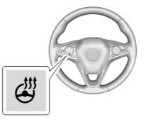
If equipped with a heated steering wheel, press to turn on or off. A light near the button displays when the feature is turned on. The steering wheel takes about three minutes to reach maximum heat.
