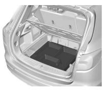
There are no attachments securing the cargo management system. Lift up on both sides to remove the cargo management system.
