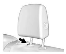
To lower the head restraint, press the button located on the top of the seatback and push the head restraint down. Try to move the head restraint after the button is released to make sure it is locked in place.
