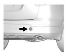
Carefully open the cover by using the small notch that conceals the rear tow eye socket.
