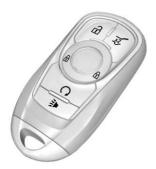
**\widehat{\mathbf{O}}**: Press to lock all doors. The turn signal indicators may flash and/or the horn may sound on the second press to indicate locking. See *Vehicle Personalization*  $\Rightarrow$  133. If a passenger door is open when  $\widehat{\mathbf{O}}$  is pressed, all doors lock. If the driver door is open when  $\widehat{\mathbf{O}}$  is pressed, all doors lock except the driver door. These settings can be modified. See *Vehicle Personalization*  $\Rightarrow$  133.
