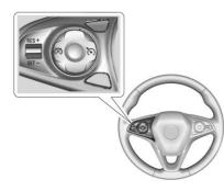
S: Press to turn cruise control on or off. A white indicator comes on in the instrument cluster when cruise control is turned on.
