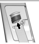
Move the height adjuster up to the desired position by pushing up on the height adjuster.
