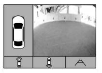
If equipped, a view of the area in front of the vehicle appears in the infotainment display. The front view shows after shifting from R (Reverse) to D (Drive) and when the vehicle is moving forward slower than 8 km/h (5 mph), or when the Park Assist system detects an object within 30 cm (12 in).
