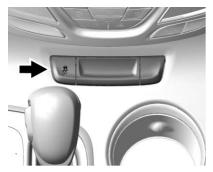
To turn off only TCS, press and release  $\frac{1}{6}$ . The traction off light (2) illuminates in the instrument cluster.
