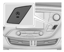
The automatic engine Stop/Start feature can be disabled and enabled by pressing the switch with the  $(\widehat{A})$  symbol. Auto Stop is enabled each time you start the vehicle.
