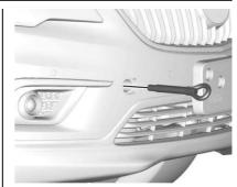
Install the tow eye into the socket and turn it until it is fully tightened.
