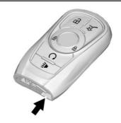
2. Separate the two halves of the transmitter using a flat tool inserted into the bottom of the transmitter.
