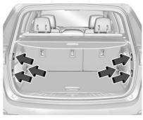
The vehicle may be equipped with six cargo tie-downs in the rear compartment.
