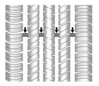
Treadwear indicators are one way to tell when it is time for new tires. Treadwear indicators appear when the tires have only 1.6 mm (1/16 in) or less of tread remaining. See *Tire Inspection*  $\Leftrightarrow$  279 and *Tire Rotation*  $\Leftrightarrow$  279.
