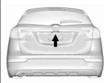
To open the liftgate, press a on the power door lock switch or press a on the RKE transmitter twice to unlock all doors. Press the touch pad on the underside of the liftgate handle and lift up.
