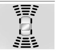
The instrument cluster may have a park assist display with bars that show "distance to object" and object location information for RPA, and on some vehicles, FPA. As the object gets closer, more bars light up and the bars change color from yellow to amber to red.
