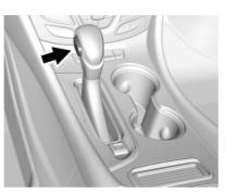
ERS or manual mode allows for the selection of the range of gear positions. Use this mode when driving downhill or to limit the top gear and vehicle speed. The shift position indicator within the Driver Information Center (DIC) will display a number next to the L indicating the highest available gear under manual mode and the driving conditions when manual mode was selected.
