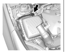
Open the hood and unwrap the electrical cord. The cord is in the passenger side of the engine compartment, near the air filter. It is shipped from the factory with a tie holding it in place. Use care in removing the tie so that the cord is not damaged.
