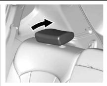
The rear outboard head restraints are designed to be folded. The head restraint can be folded backward to allow for better visibility when the rear seat is unoccupied. To fold the head restraint, press the button on the side of the head restraint.
