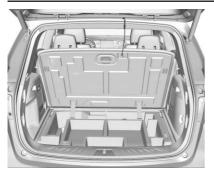
Remove the load floor hook from the holder and hook to the weatherstrip above.
