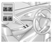
Power windows work when the ignition is on, in ACC/ACCESSORY, or when Retained Accessory Power (RAP) is active. See *Retained Accessory Power (RAP)* ⇔ 179.
