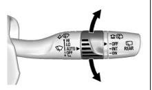
**AUTO :** Move the windshield wiper lever to AUTO. Turn the band on the wiper lever to adjust the sensitivity.
