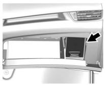
The instrument panel fuse block is in the glove box. To access the fuses, open the fuse panel door from the passenger side by pulling it out. To reinstall the door, insert the tabs on the top of the door into the console first, then push the door back into its original location.
