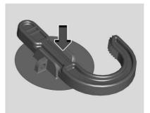
2. Push down on the other side of the load floor hook to lock into place.
