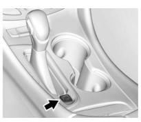
The Electric Parking Brake (EPB) switch is on the center console. The EPB can always be activated, even if the ignition is off. To prevent draining the battery, avoid repeated cycles of the EPB when the engine is not running.
